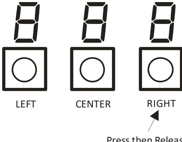
2. Press and release the Right Button (this will cycle through the menus in one direction. Pressing the Left Button would cycle through the menus in the opposite direction. For this example, the right button will be used).
