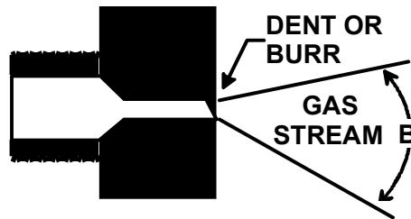
A dent or burr will cause severe deflection of the gas stream.
