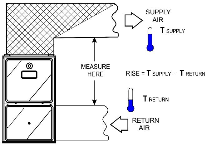
3. Subtract the return air temperature from the supply air temperature to determine the air temperature rise. Allow adequate time for thermometer readings to stabilize.
