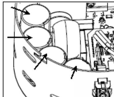
7. Locate the 3-circuit connector in the control/end bell. Using an ohmmeter, check the resistance between each terminal in the connector. If the resistance is  $100\text{k}\Omega$  or greater, the control/end bell is functioning properly. Replace the control/end bell if the resistance is lower than  $100\text{k}\Omega$ .
