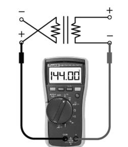
If meter reads approximately 96 volts - the primary to secondary are in phase - if reads approximately 144 volts out of phase - reverse low voltage wires.
